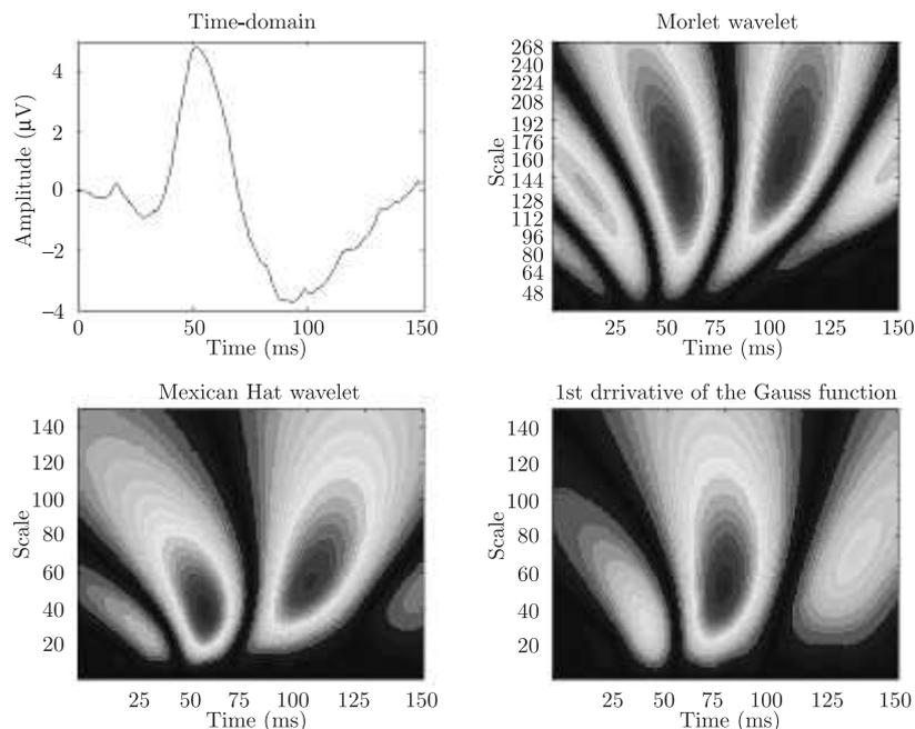
Fig. 3. Comparison of CWT results for the same PERG waveform (with three different wavelets, after Ref. 14)
